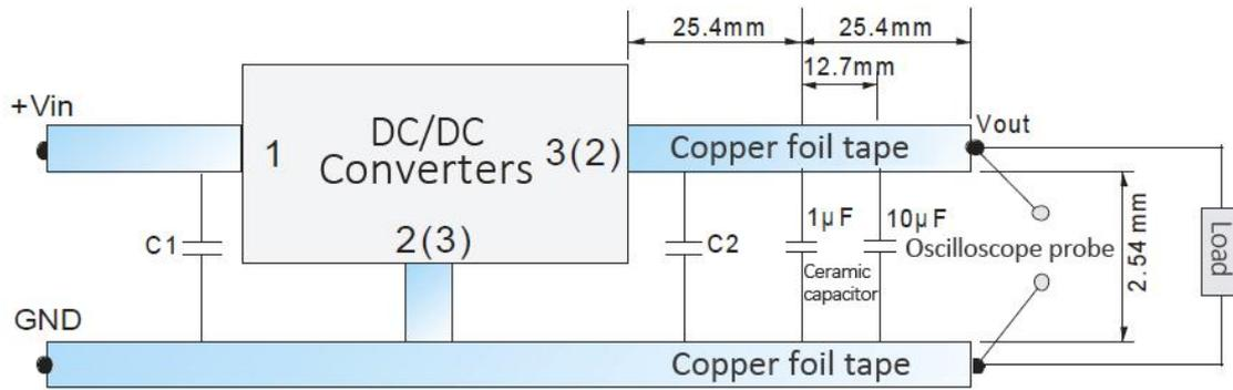
Diagram 2-1 Parallel cable measuring method
