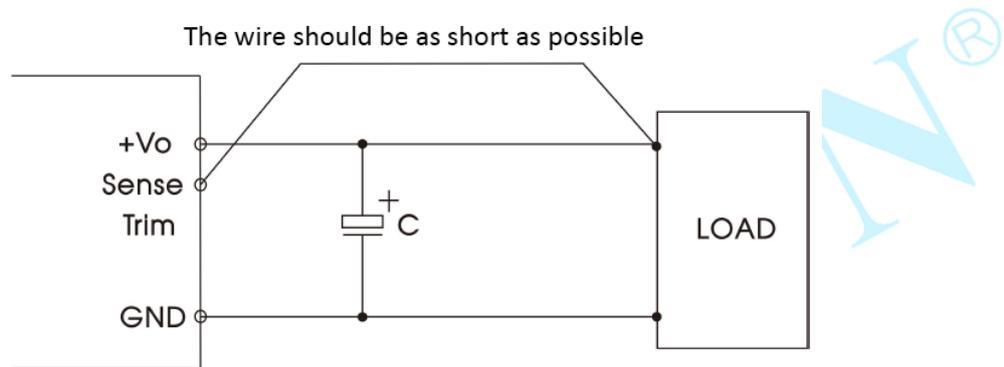
Diagram 3-9 Sense pin remote compensation application
