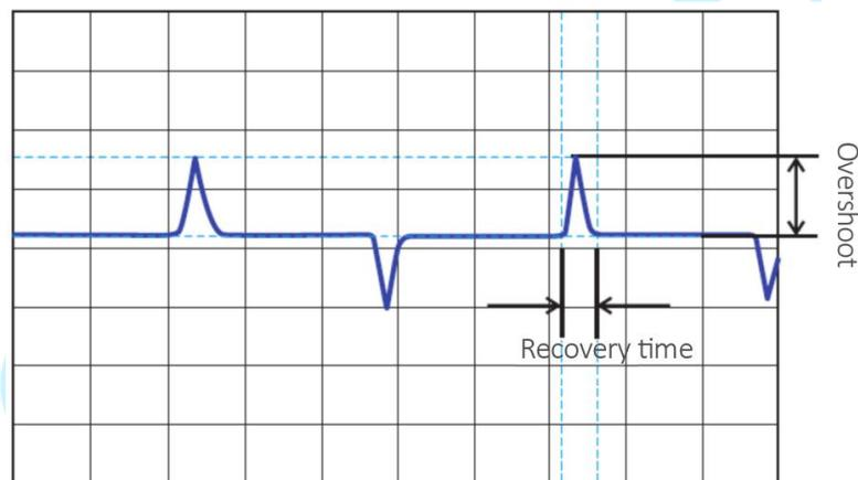
Diagram 2-4 Waveform of dynamic load Test
