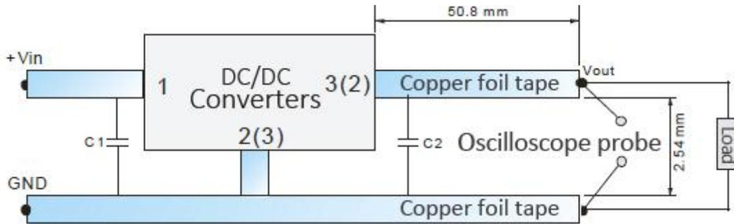
Diagram 2-3 Connection of dynamic load Test
