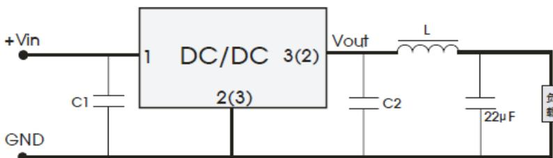
Diagram 3-5 Recommended circuit reducing ripple & noise
